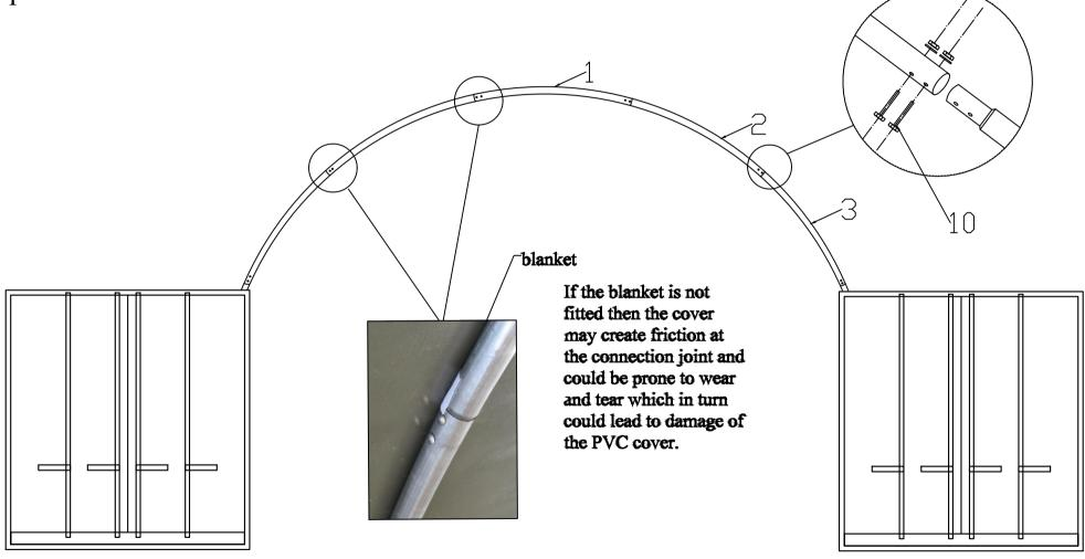
If the blanket is not fitted then the cover may create friction at the connection joint and could be prone to wear and tear which in turn could lead to damage of the PVC cover.
